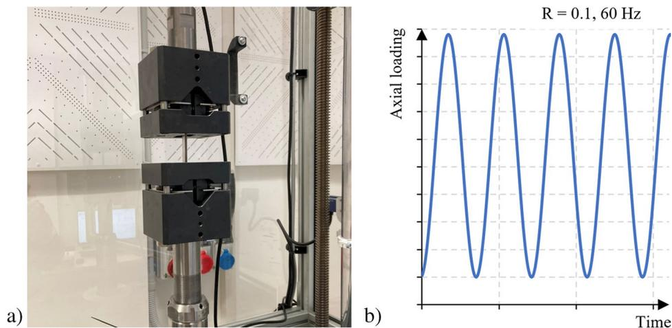
of experimental data points for the non-linear fitting of the S–N fatigue curves. A total of 15 samples, sized as shown in Fig. 3, were tested, with 2–3 specimens tested at each load increment. The Wöhler curve is fitted according to Eq. (1) [31]:
