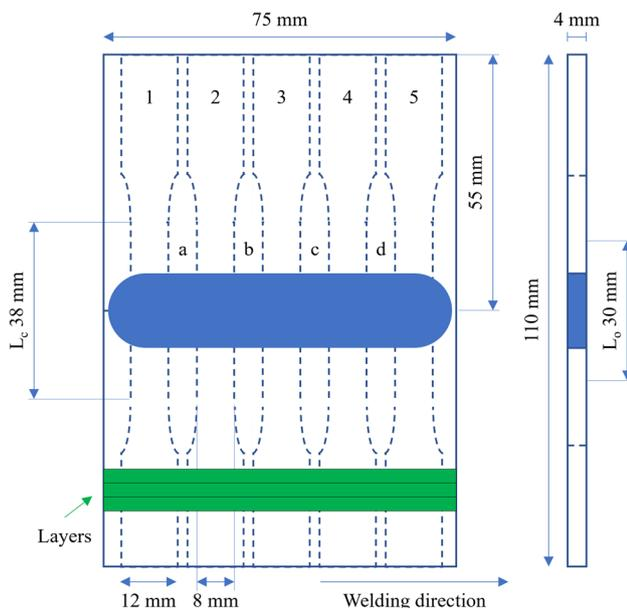
**Fig. 3** Sketch of the FSW welds, tensile, and metallographic samples with the build direction of the printed layers (green colored)
