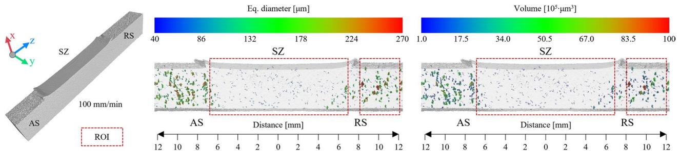
**Fig. 12.** 3D X-ray computed tomography: distribution, equivalent diameter, and volume of the pores in the BM and FSW areas for the joint obtained with a welding speed of 100 mm/min. Data from the two ROIs are further analyzed in Fig. 13
