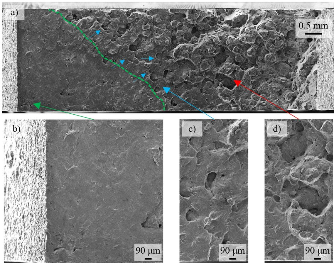
**Fig. 19** Fracture surface and high magnifications of the HT FSW joint obtained with a welding speed of 100 mm/min after fatigue tests: **a** general overview of the fractured BM, **b** detail of the crack initiation region, and **c**, **d** detail of the final fracture region
