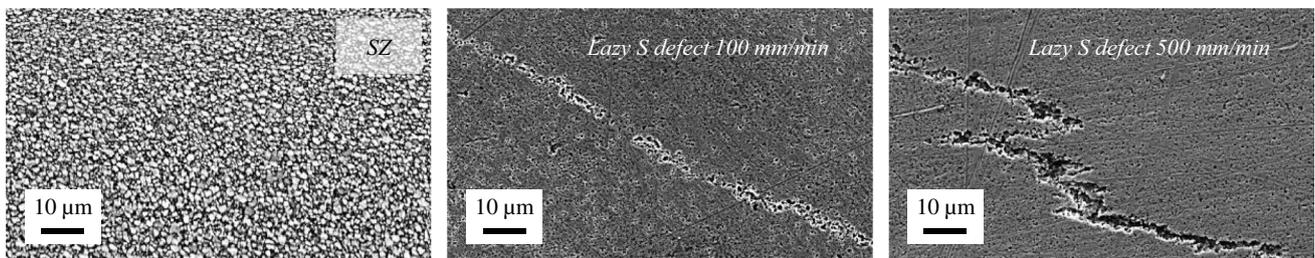
**Fig. 9** SZ microstructure and lazy S defect in the FSW joints of Fig. 8
