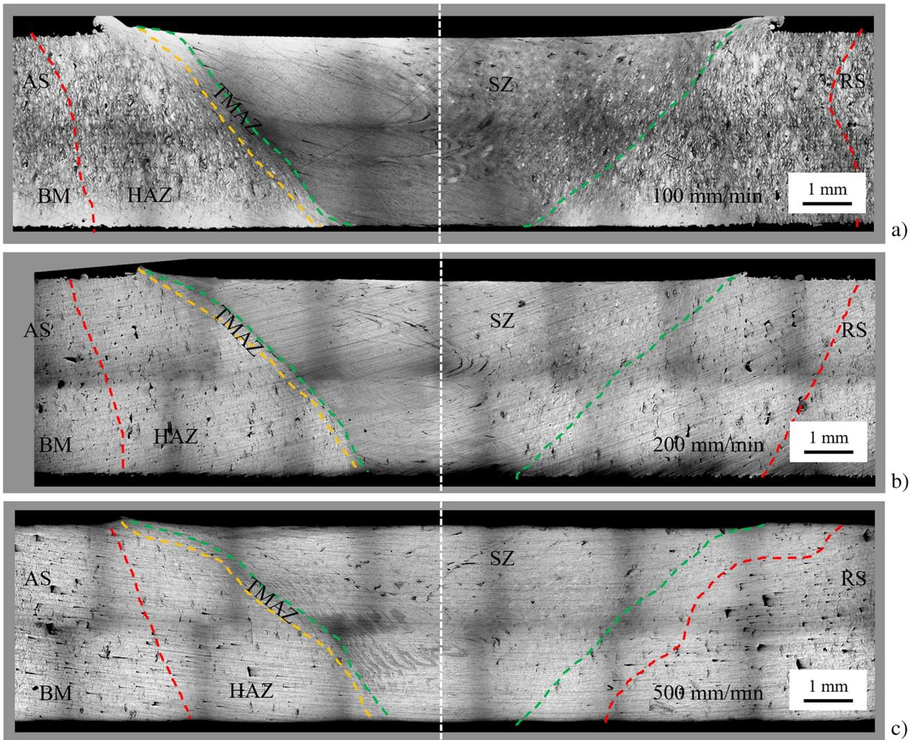
**Fig. 8** Cross-section of the FSW joints with the variation of the welding speed: **a** 100 mm/min, **b** 200 mm/min, and **c** 500 mm/min. The three images have been obtained from the stitching of a collection of optical images
