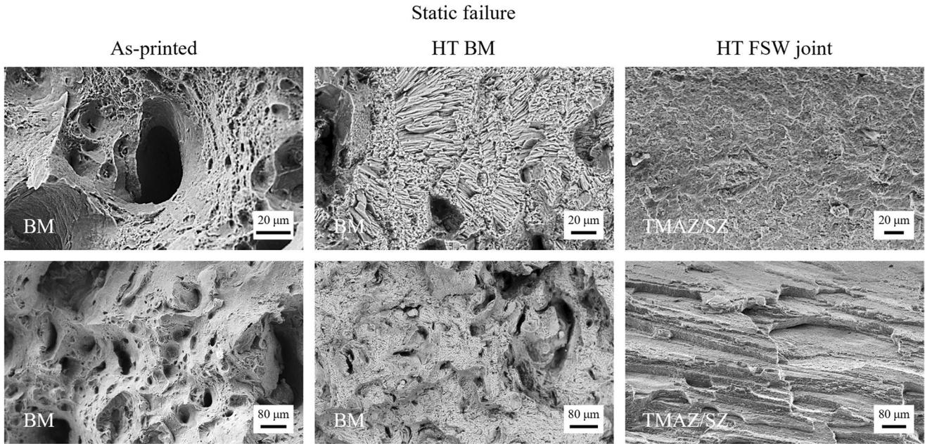
Fig. 16 High magnification of significant details of the fracture surfaces
