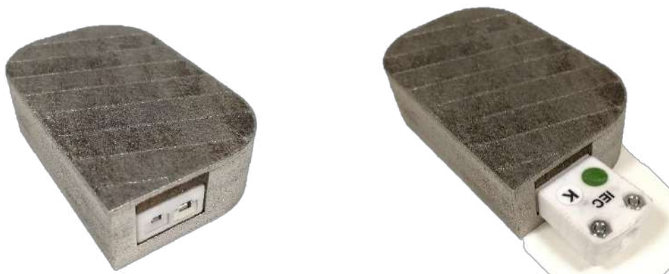
Figure 4. Sample released in final configuration with integrated sensor and external connection.
