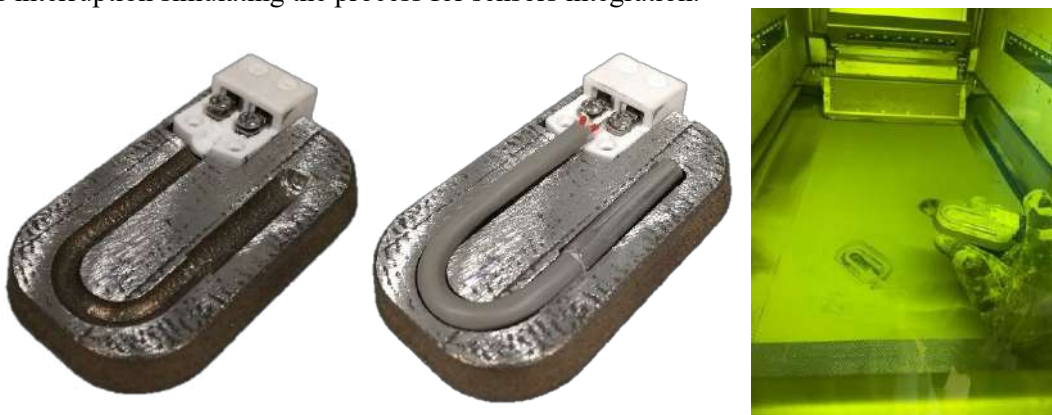
Figure 3. Internal view of the sample built with In718 and embedded PT100 sensor with ceramic connector USHX and electronics embedding operations.
