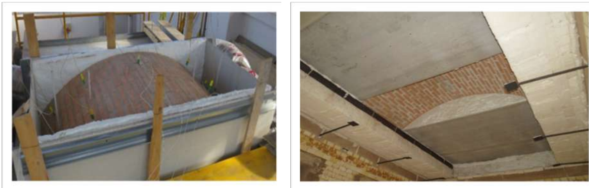
Figure 1 – The barrel vault subjected to elevated temperatures
