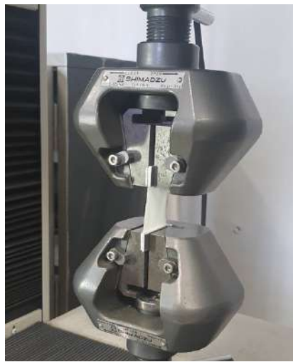
Figure 2. Membrane sample during the tensile test.
