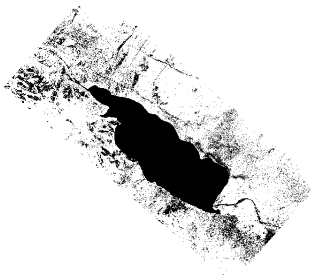
Figure 1. Masked raster showing valid vegetated pixels after NDVI thresholding ( NDVI > 0.30 ) and water removal.
