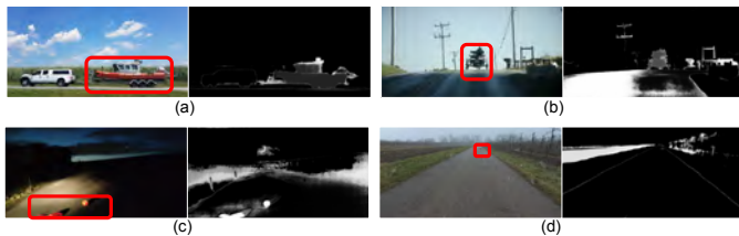
Fig. 15: Failure Cases: (a, b) Mask2Anomaly fail to segment trailer or carriage as they have a similar appearance as car or bus. Mask2Anomaly struggle to perform well in poor illumination (c) and weather conditions (d). The white region represents the anomalies that are enclosed in red boxes.
