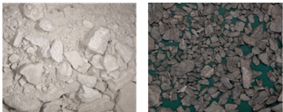
(a) The material as it is extracted from the TBM
