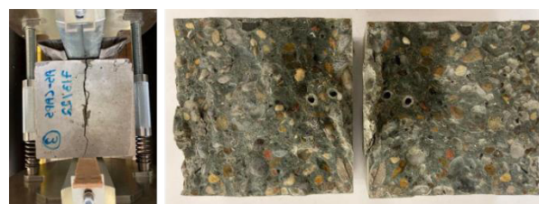
Fig. 8. Splitting the cube specimens to count the amount of broken capsules in a certain crack plane (note: the darkest concrete surface is the area covered by WRA)
