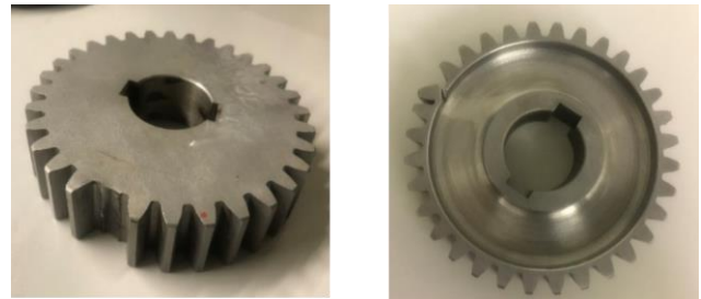
Figure 6 Failures on standard (left side) and thin-rim (right side) gears subjected to fatigue tests [25].
