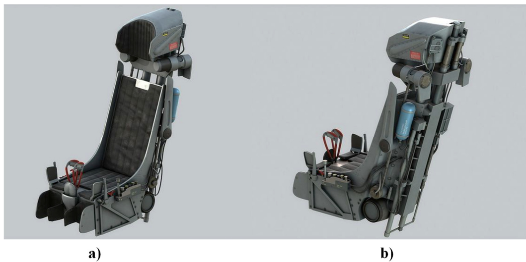
Figure 1. Fourth-generation k-39 ejection seat. (a) Front view; (b) rear view.
