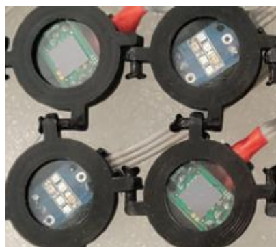
Figure 3. Details of SiPMs (top left and bottom right) and LEDs (top right and bottom left) for diffused optical tomography/functional near-infrared spectroscopy (DOT/fNIRS).
