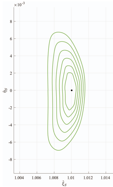
Fig. 6.2 SEL2 QPLOs with initial analytical A_y = [3, 8] \times 10^5 km at \mathcal{E}_1 , SE synodic RF
