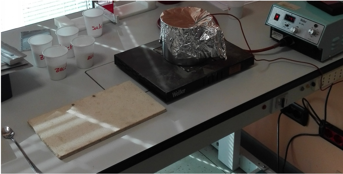
Figure 3.1: Preparation of the semi-solid agar mixture using an electric hotplate and a temperature probe.
