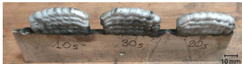
Figure 2. Semi-continuous dot-by-dot tests
