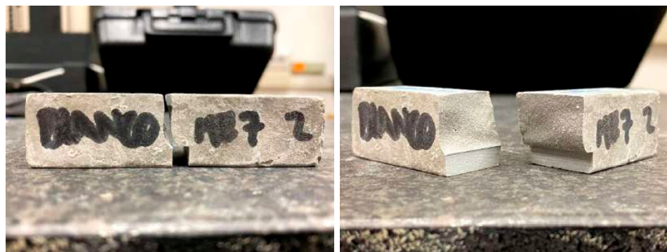
Figure 9. Linear crack path and smooth fracture surface. Plain cement (OPC) at 7 days.
