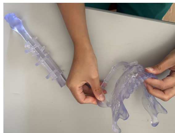
FIGURE 6 Participant interacting with 3D printed cutting guides and anatomical models.
