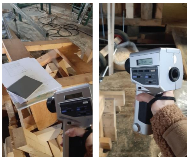
Figure 5. Field luminance measurement is used to calculate the light reflectance of real materials for simulations [44].
