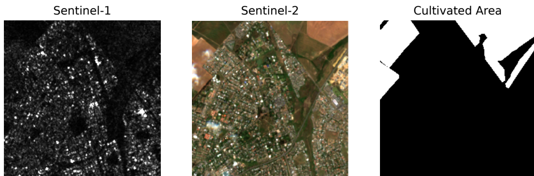
Figure 3.8: Crop field segmentation task. From left to right: a Sentinel-1 image (VV polarization), the corresponding Sentinel-2 RGB image, and the ground truth binary mask where cultivated areas are highlighted in white.
