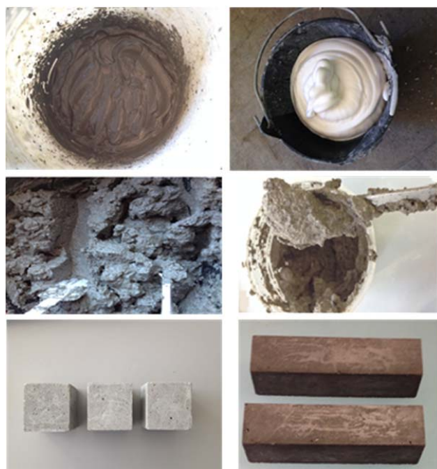
Fig. 1 Preparation of extrudable foamed concrete specimens
