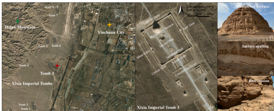
Fig. 2. Case study overview. (a) Distribution map of the Xiaxia Imperial Tombs earthen heritage complex; (b) Plan of Xiaxia Imperial No. 3 tomb; (c) Current surface erosion features of No. 3 tomb.
