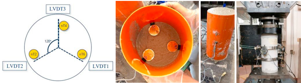
Fig. 2. Instrumentation of the pilot mortar specimen and test setup.
