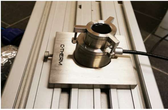
Fig. 2. Image of the thermal conductivity sensor. The nanocomposite in the liquid phase (black material) is inside the mold (upper part of the sensor). The cylindrical part at the bottom is the sensor, which measures the thermal conductivity.
