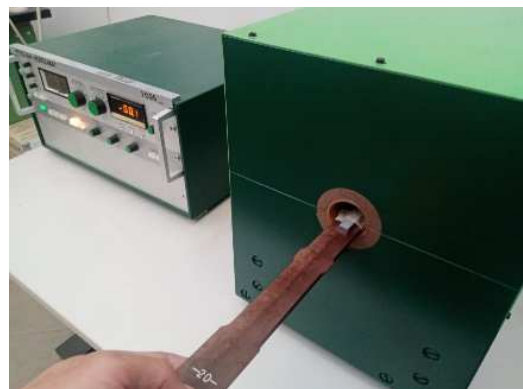
Fig. 4 - Specimen insertion in the coercimeter coil
