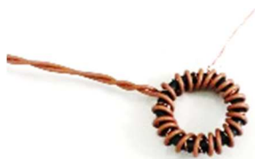
Fig. 5 - FeSi2.9 Toroid: size and shape not fully compliant with the IEC 60404 series standards
