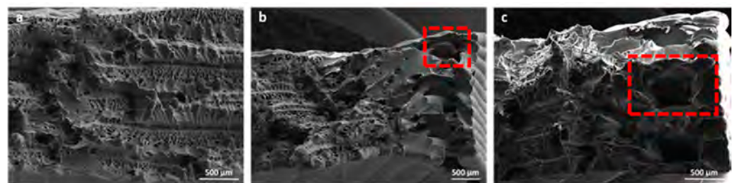
Figure 12. Explanatory SEM images of the fractured surfaces: (a,b) from specimen tested at 0.5 mm/min and (c) from specimen tested at 10 mm/min. Red boxes indicate the possible crack initiation site. Original images, from Figures S1–S3, are available in the Supplementary Materials.
