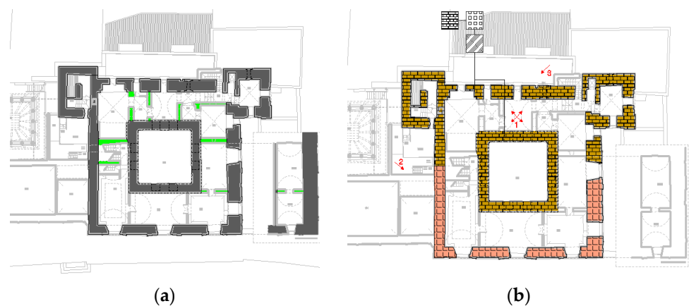
Figure 21. Identification of the structure of the Tower on level H (height 28.70 m): (a) hypothesized vertical load-bearing structure; (b) hypothesized materials.
