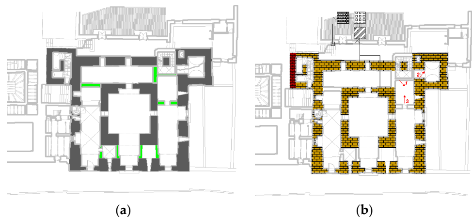
Figure 19. Identification of the structure of the Tower on level F (height 23.60 m): (a) hypothesized vertical load-bearing structure; (b) hypothesized materials.
