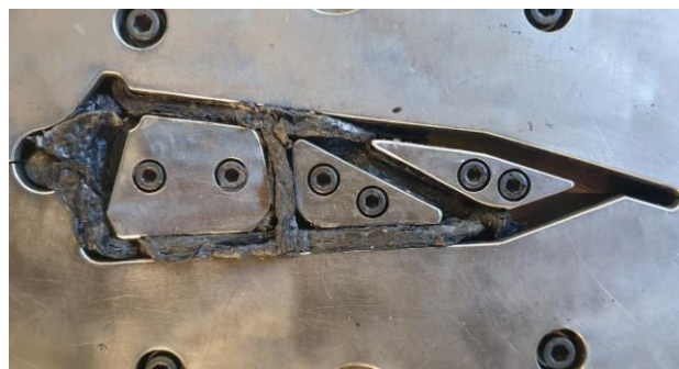
Figure 6.3. Lower tool cavity partially filled. The image refers to the procedure B, where only a portion of the mold surface is filled.
