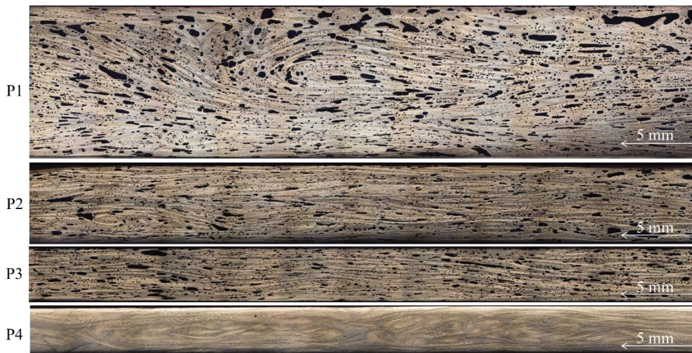
Figure 3.6. Micrography of the partially molded plates (P1-P3) and of the fully molded plate (P4).
