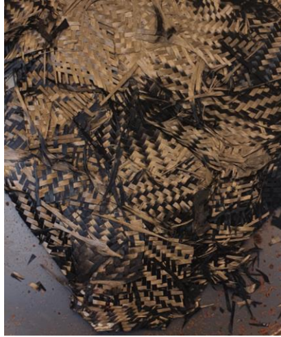
Figure 3.11. Peeling analysis of the CP100 plate.
