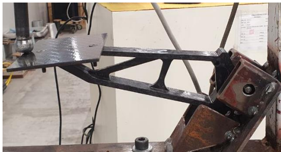
Figure 6.6. Testing frame: a) Load and constrain condition (dimensions are expressed in mm); b) test set-up; c) detail of the hinge area; the screw reproduces the end of the pedal stroke.
