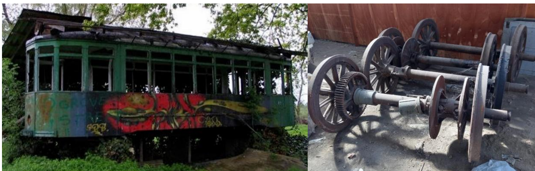
Figure 1: Carbody of Tram 614 and Wheelset of the 2700 series before restoration.
