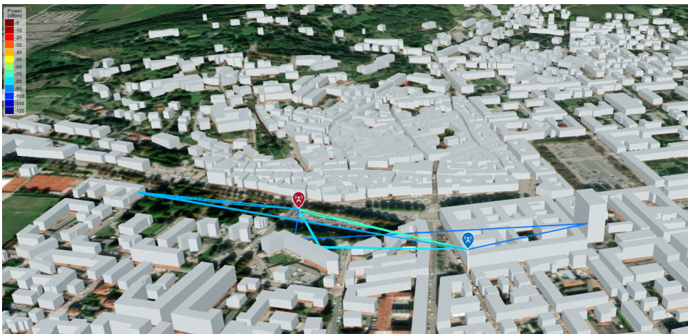
Fig. 6.3 Visualization of the ray-tracing output, depicting the receiver with a blue point and the transmitter with a red point. Each ray represents reflections and diffractions of the signal, with varying colors indicating different power levels.
