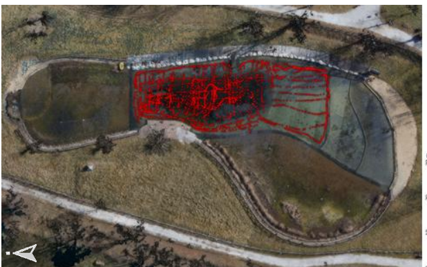
Figure 5. Trajectory of bathymetric points acquired with the Blue Boat USV within the Biolago di Caraglio
