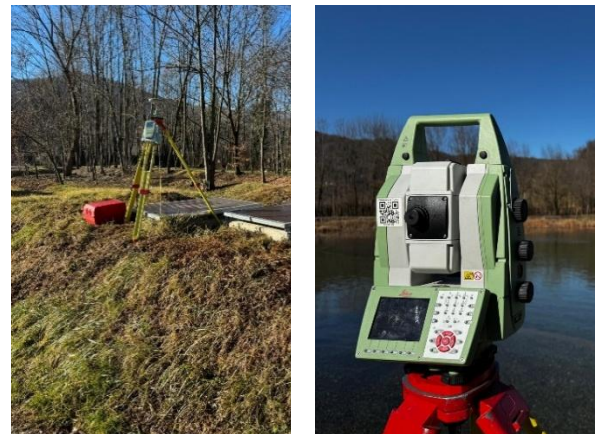
Figure 2. Instruments used for the topographic survey, Leica System 1200 GNSS receiver (left), Leica Nova MS60 Total Station (right)
