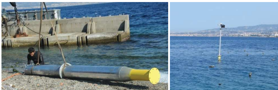
198 199 Figure 2 – Spar hull model before (left) and after (right) installation, sustaining the parked turbine model 200 [29]
