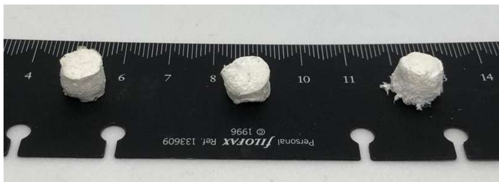
Figure 25. Hydrogels obtained after the freeze-dry process. From left to right: MCHIT, MCHIT3 and MCHIT5
