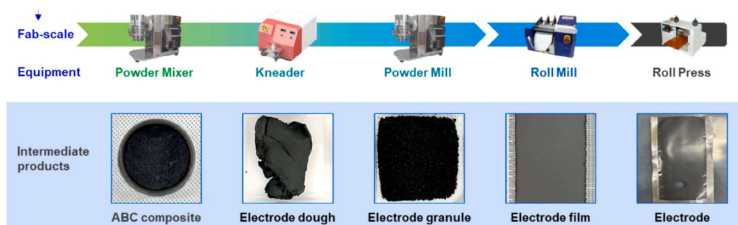
FIGURE 2 | Dry electrode manufacturing steps and equipment for fabricating a LIB cathode electrode composed of polytetrafluoroethylene (PTFE) binder, single-crystal \text{LiNi}_{0.8}\text{Co}_{0.1}\text{Mn}_{0.1}\text{O}_2 (NCM811) active material, and carbon black (CB, Super P) and carbon nanotube (CNT) conductive agents [39]. Reproduced (Adapted) with permission, Copyright 2024, Elsevier.
