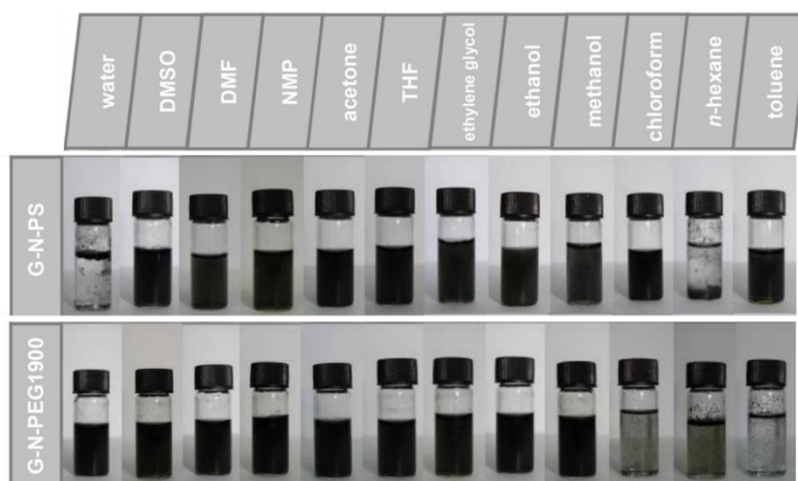
Figure 1.5 Photographs of polystyrene and poly(ethylene glycol) functionalized graphene nanosheets (G-N-PS and G-N-PEG1900) in various solvents. Reproduced with permission from [89]. Copyright 2010, American Chemical Society.
