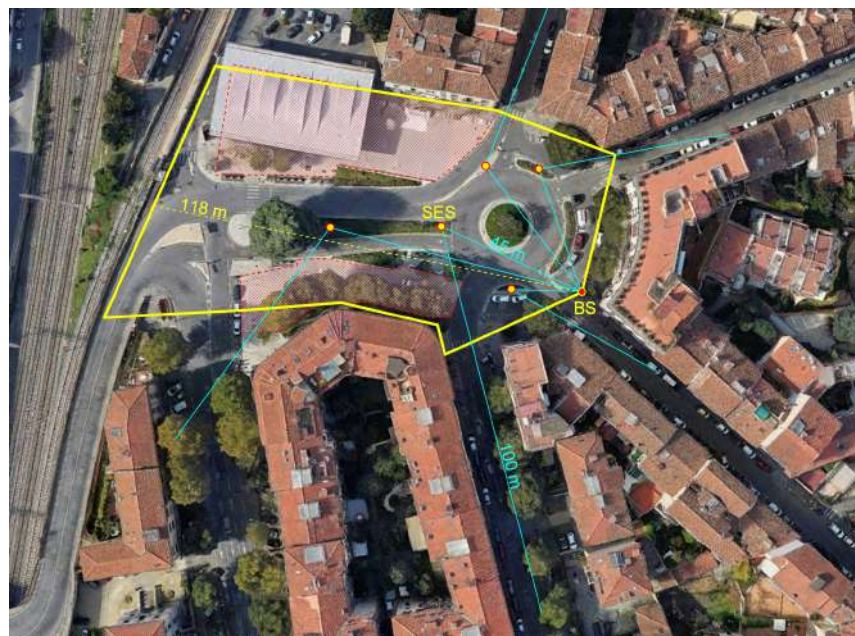
Figure 1. A possible scenario of application 5G. The yellow area is the LOS area covered by the base station (BS), represented by a red dot. The hatched red area represents the market area. The yellow-red circled dots identify the location of existing light poles where curved SESs can be mounted.
