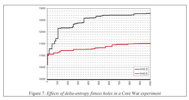
Lastly, Figure 7 shows the score attained by the best warrior against the test hill during the 1,000 generations of the experiment. The effect of a delta-entropy fitness hole (h=0.3) was compared against the standard selection mechanism (no hole, h=0.0). All the other settings were identical and are described above. The practical effect of the delta-entropy fitness hole is evident.
