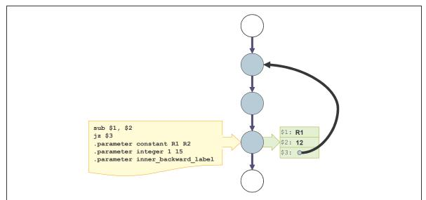
Figure 3: A short program with a one node implementing a 2-line, 3-parameter macro. The highlighted node contains the actual values of the parameters: the constant string R1, the integer number 12, and a reference to a preceding node.
