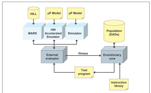
Figure 1:  $\mu$ GP system architecture. The characteristics of the assembly language are stored in the instruction library. The evolutionary core evolves a population and may exploit different fitness functions for different problems through the external evaluator.
