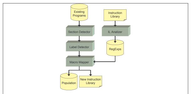
Figure 4: Assimilation Process. The existing programs are analyzed using different heuristics, and the Instruction Library transformed in a set of regular expressions in order to discover a possible mapping. The result is a Population and a new Instruction Library.
