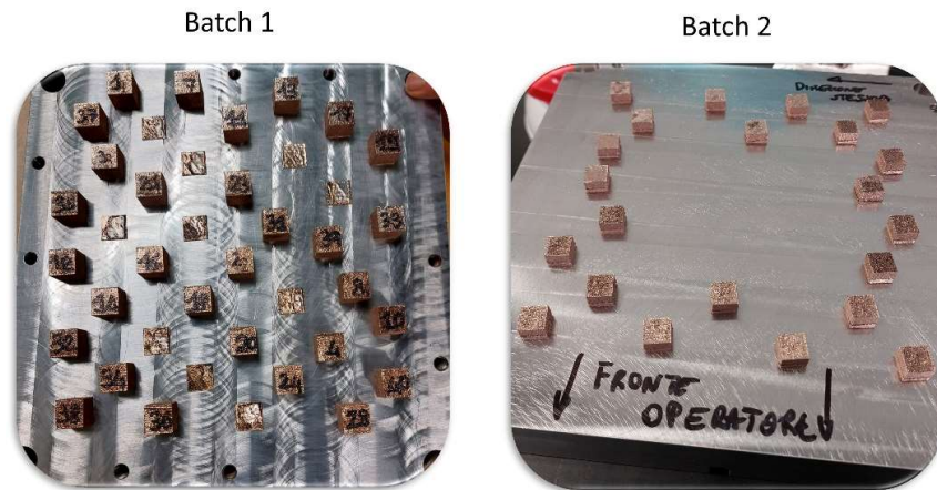
Figure 37. Batch 1 and 2 of CuNi2SiCr samples produced by medium-power red laser machine.
