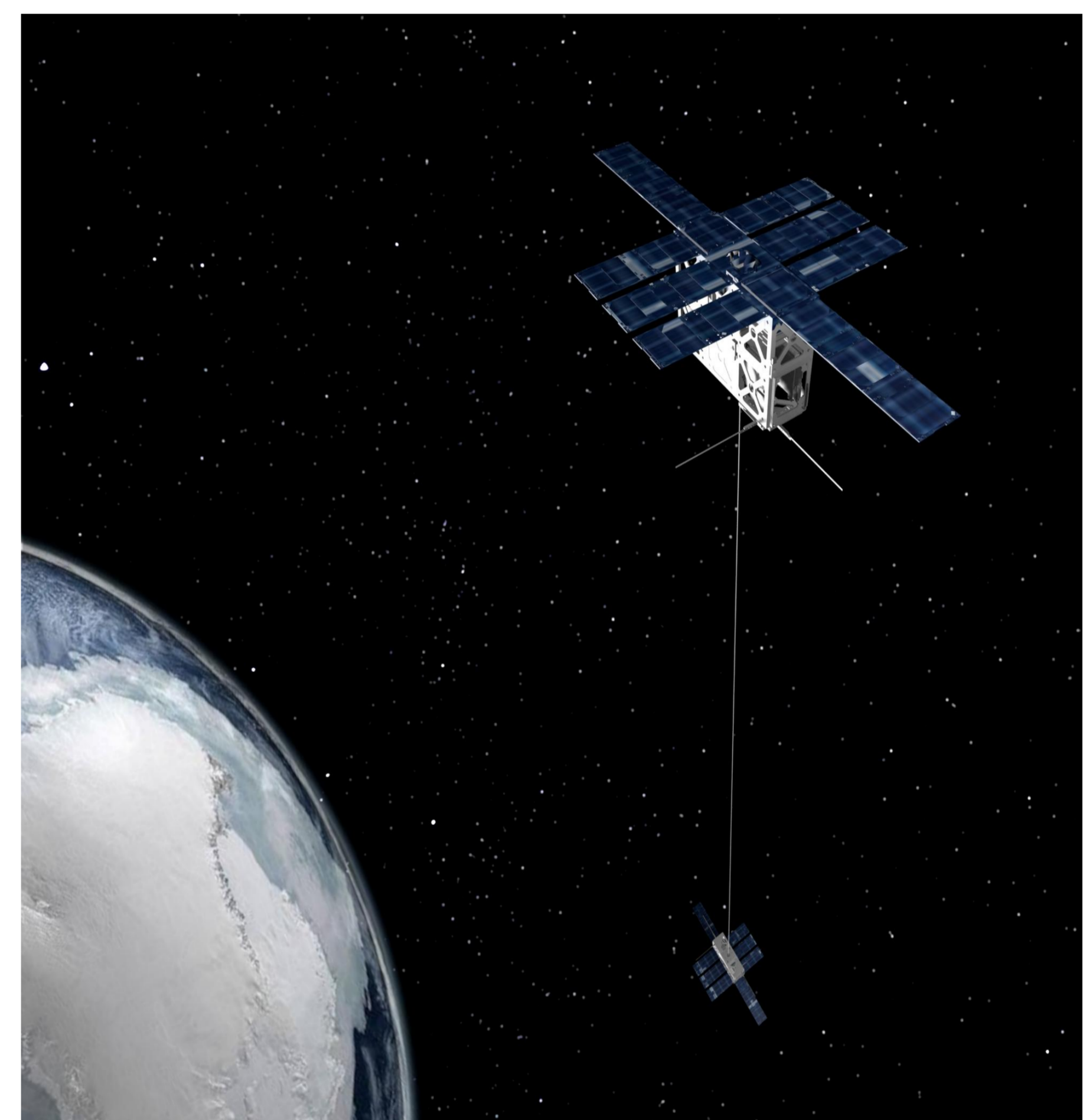
Fig. 3 Tethered system stabilized in the cross-track direction by aerodynamic forces. Credit. ASTRADORS lab
