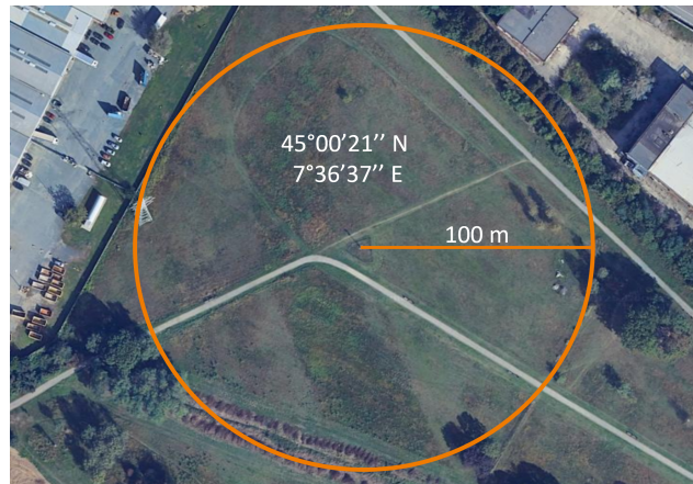
Fig. 2.1 Google Earth picture of the site, with the 100 m radius free of obstacles around the station, positioned in the centre of the red circle. The coordinates of the station are reported in the picture. It is worth mentioning that all trees have been cut in the area internal to the red circle, according to the WMO prescriptions, in order to reduce uncertainties in the data representativeness and measurement errors.
