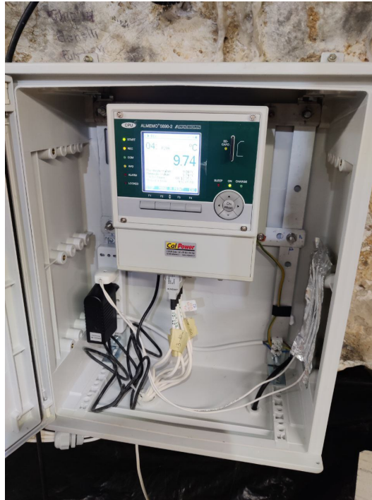
Fig. 6.2 Example of datalogger installation in a monitoring point of the Bossea cave. On the internal wall, on the right, it is visible the electrical heater used to reduce the relative humidity and avoid water condensation on the datalogger.
