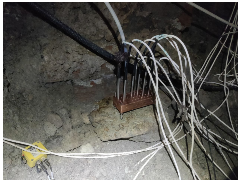
Fig. 6.6 Comparator block exposed to free air during verification at Porfiroidi.
