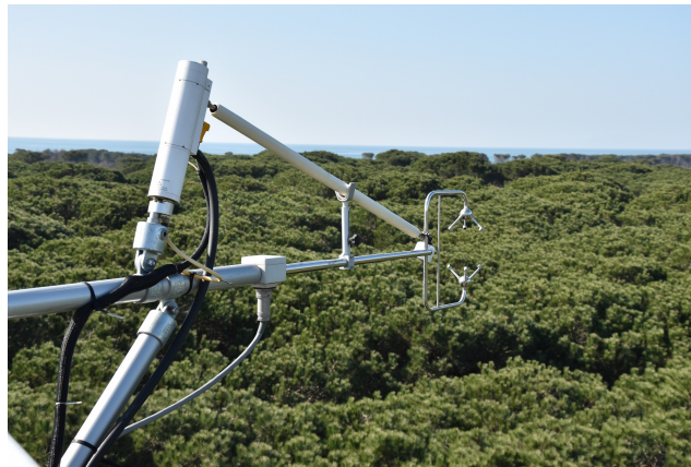
Fig. 5.3 Configuration of a gas analyzer coupled with a sonic anemometer used for EC measurements.
