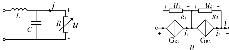
(a) Proposed circuit model for MOA (b) Proposed dynamic nonlinear resistance defined by (3-41)
