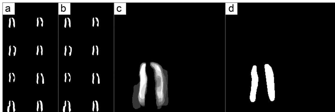
Figure 5. (a) Binarized SoftMax outputs from eight separately trained models. (b) Post-processed SoftMax. (c) Averaging of the 8 SoftMax results in a probability map. (d) Post-processing of the probability map (thresholding at 0.6 and morphological operations).
