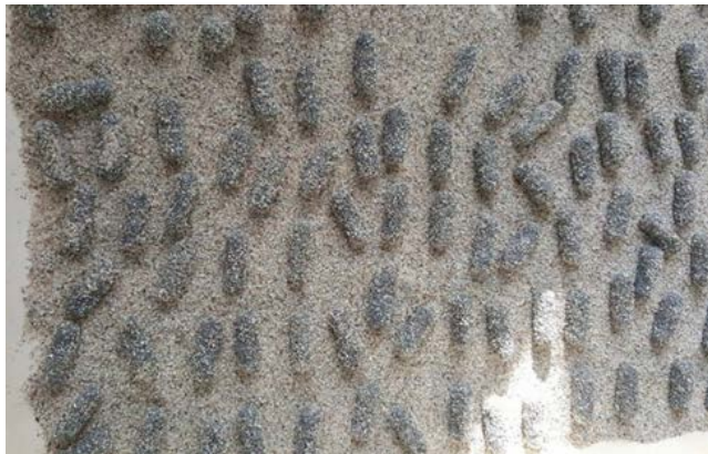
Fig.2. Epoxy resin and sand coating on pharmaceutical capsules.
