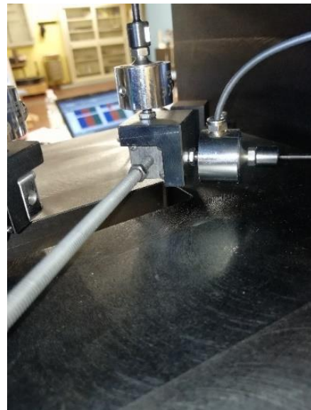
Figure 43: Rod pusher setup for compressive force calibration
