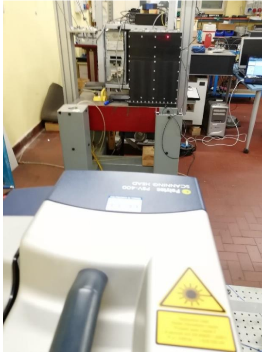
Figure 37: Using SLDV to find the modes of the test rig structure
