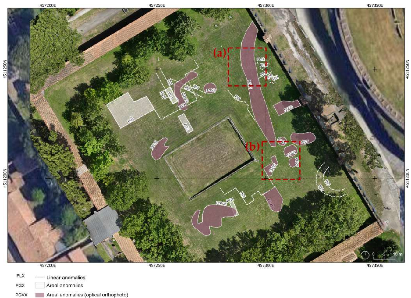
FIGURE 8 | Totality of anomalies detected in Palestra Grande . The ones in purple are detected in the RGB orthophoto. Red squares (a), (b) indicate areas corresponding to zoomed-in images of specific anomalies, highlighting vegetation anomalies already detectable in the RGB orthophoto.
