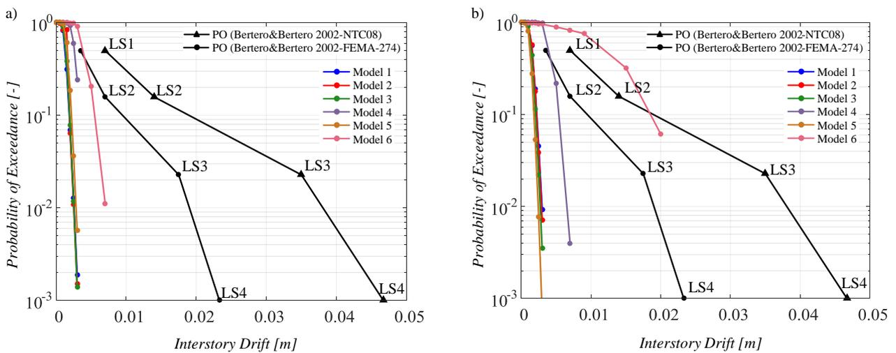
Figure 6. Exceeding bivariate probabilities at the substructure-joint 29, related to configuration with (a) and without (b) the connecting beams.
