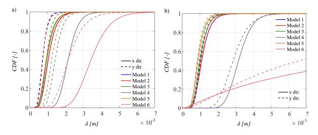
Figure 3. Lognormal monovariate PDFs at the substructure-joint 29: structure with (a) and without (b) the connecting beams.
