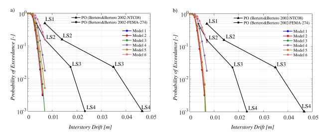
Figure 5. Exceeding bivariate probabilities at the 4th story, related to configuration with (a) and without (b) the connecting beams.
