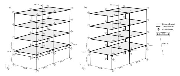
Figure 1. Base-isolated structure configurations with(a) and without(b) the beams connecting the substructure columns.
