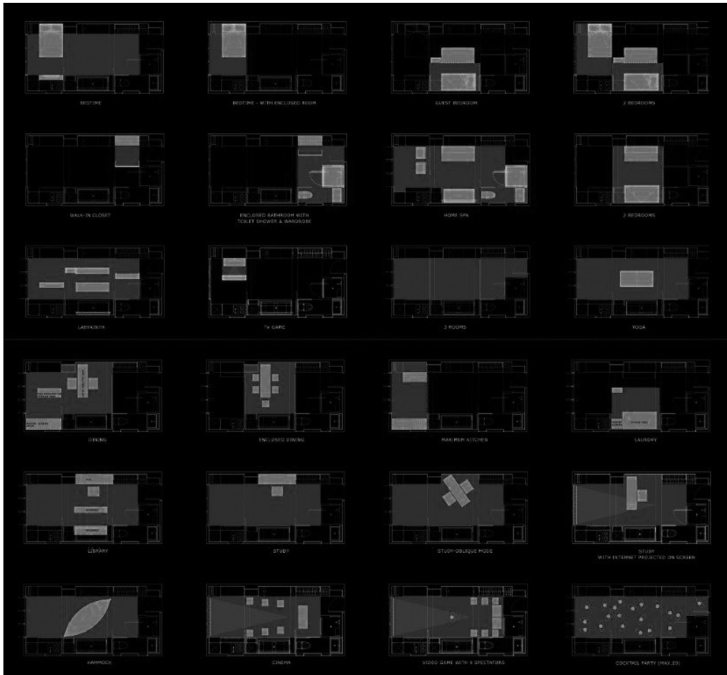
Fig. 3 - The 24 configurations of the Domestic Transformer designed by Gary Chang (2007). Photo courtesy of Edge Design Institute Ltd.
