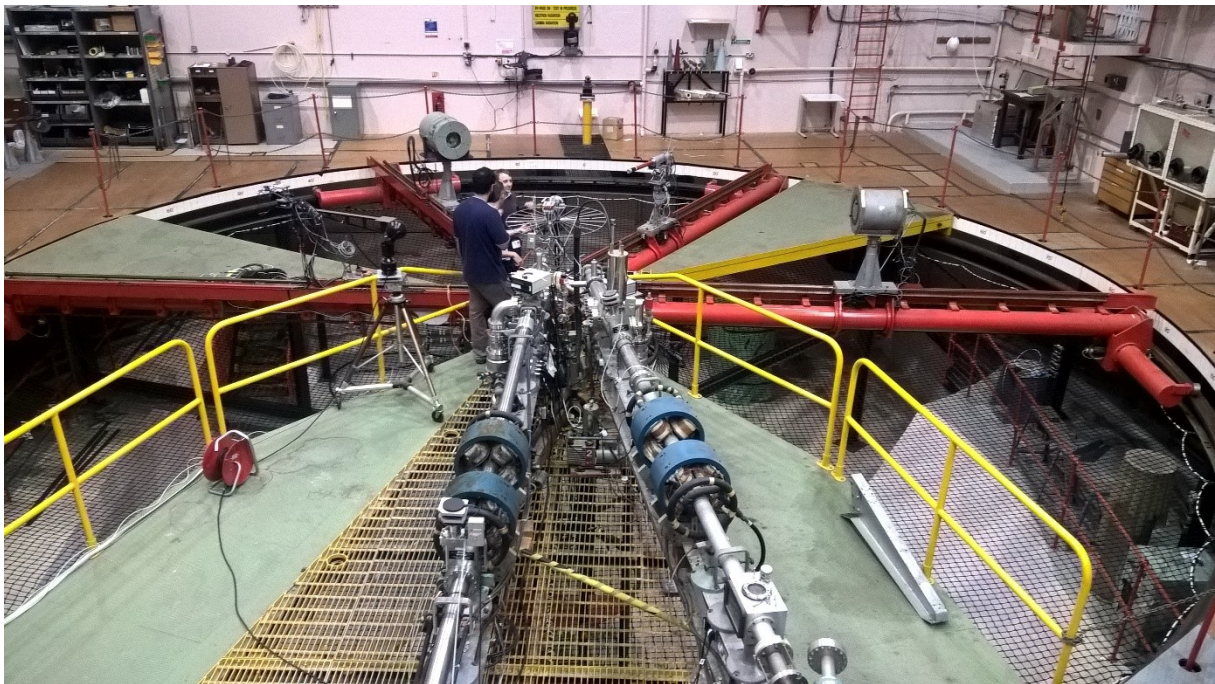
Fig. 1 Experimental hall inside the Chadwick facility. The NG is located in the centre of the hall. The two long counters and the NE-213 scintillator are situated above the red rails in the centre of the above image.
