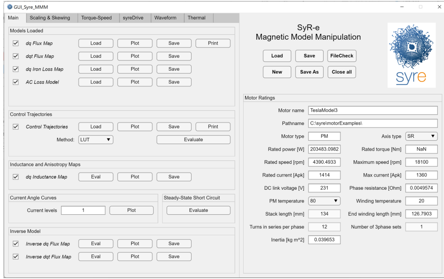
Fig. 2.3 MMM GUI of SyR-e for magnetic model manipulation.
