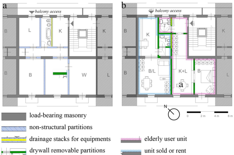
Figure 3. Figure 3a shows the 90 m2 dwelling in the original state, while 3b shows a possible transformation in scenario B2.
