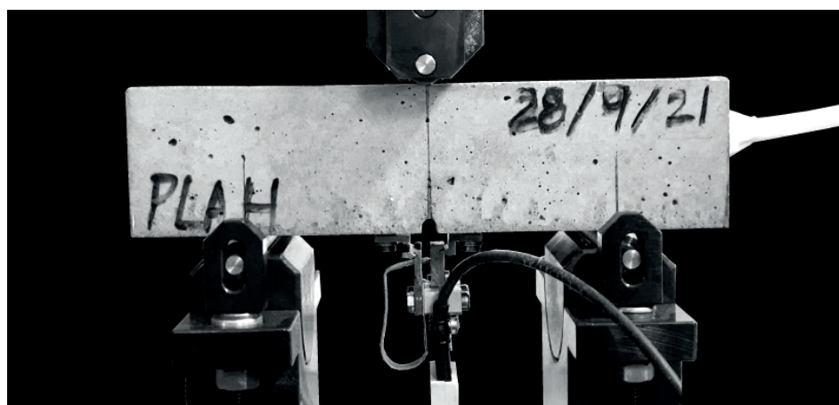
Figure 2. Three-point bending test with CMOD device.
