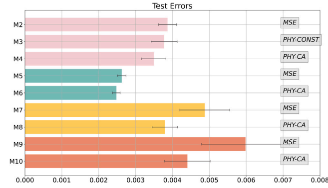
Fig. 7. Comparisons of test error by different model on D_1 data set. Vertical axis represents different models M2 to M10 with abbreviations of the employed loss function indicated in gray boxes on the right: “MSE” denotes the vanilla DNN, “PHY-CONST” denotes the PINN with constant hyperparameter ( \lambda_{LM} = \lambda_{max} ), and “PHY-CA” denotes the PINN with cyclical annealing scheduler. Results in red bars are yielded from models (M2, M3, M4) trained on 60% of data ( \sim 9k ) without BN. Results of similar models but trained with BN (M5, M6) are shown in green. Yellow (M7, M8) and orange (M9, M10) bars show the results of models with BN but trained only on 20% of data ( \sim 3k ) and evaluated on 40% ( \sim 6k ) and 80% ( \sim 12k ) of data, respectively. All the results are averaged over multiple seeds with error bars representing the standard deviation. (For interpretation of the references to color in this figure legend, the reader is referred to the web version of this article.)
