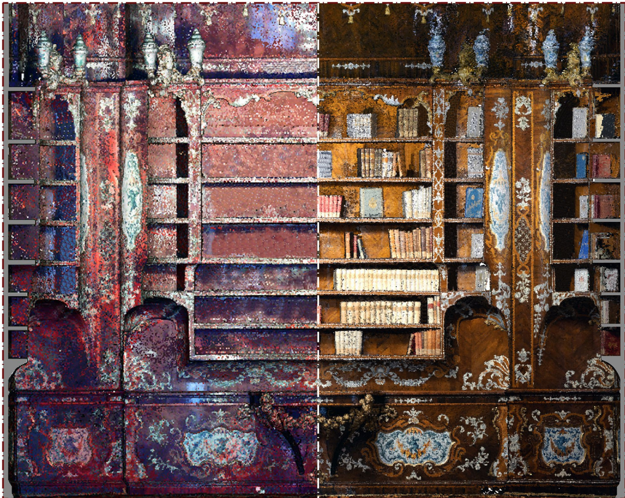
Figure 9. The front side of the library. On the left is the range-based data, and on the right, is the point cloud from photogrammetry.
