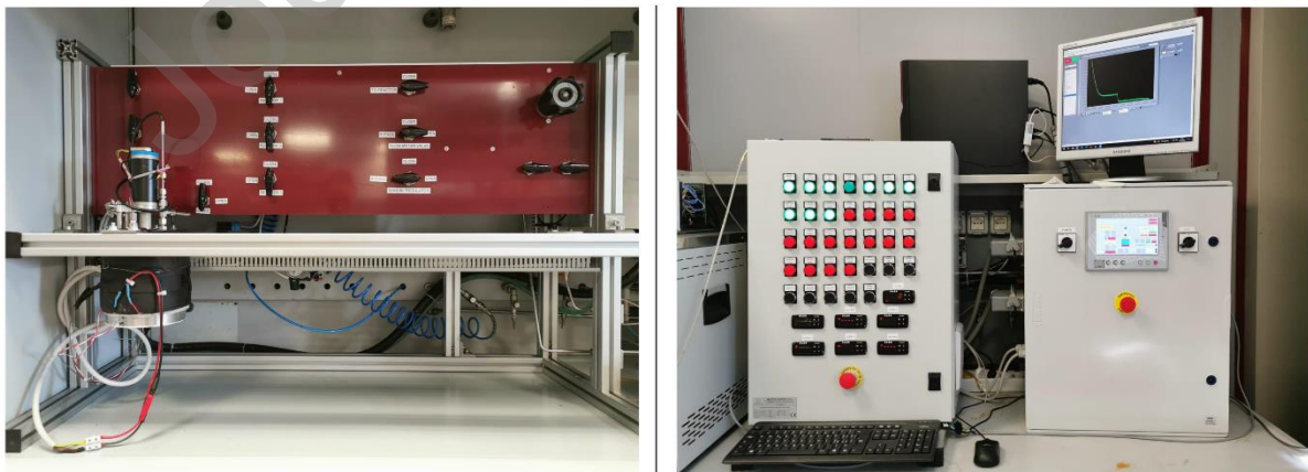
Fig. 4. Picture of the multiple-reactor apparatus (left panel); picture of the PLC control system (right panel). Modified with permission from Ref [37] Copyright (2017) ACS.
